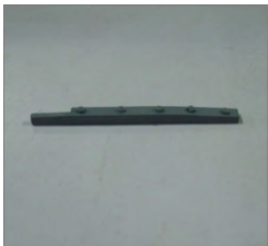
(1) Periscope Bolt Detail B (Long) BRA006-415R
