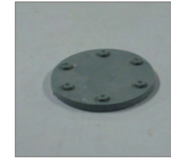
(1) Rear Crew Compartment Vent BRA006-416R
