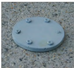
(1) Rear Crew Compartment Vent BRA006-416R
