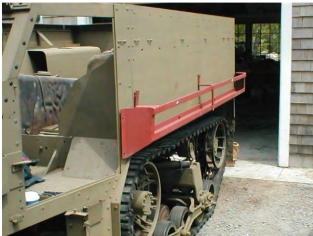
Bend tabs to fit on holes in front of halftrack.
