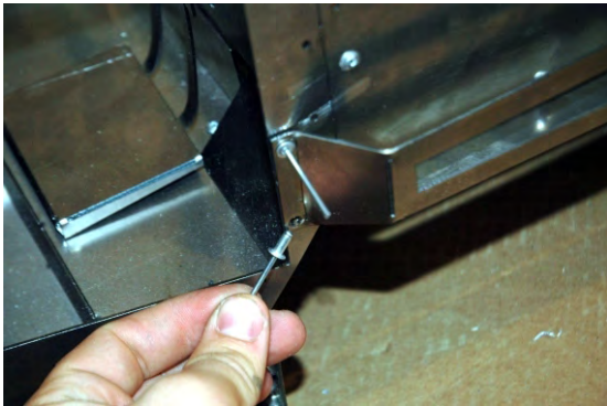
Bend tabs to fit on holes in front of halftrack.
